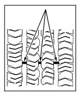
One way to tell when it is time for new tires is to check the treadwear indicators, which will appear when your tires have only 1/16 inch (1.6 mm) or less of tread remaining. Some commercial truck tires may not have treadwear indicators.
